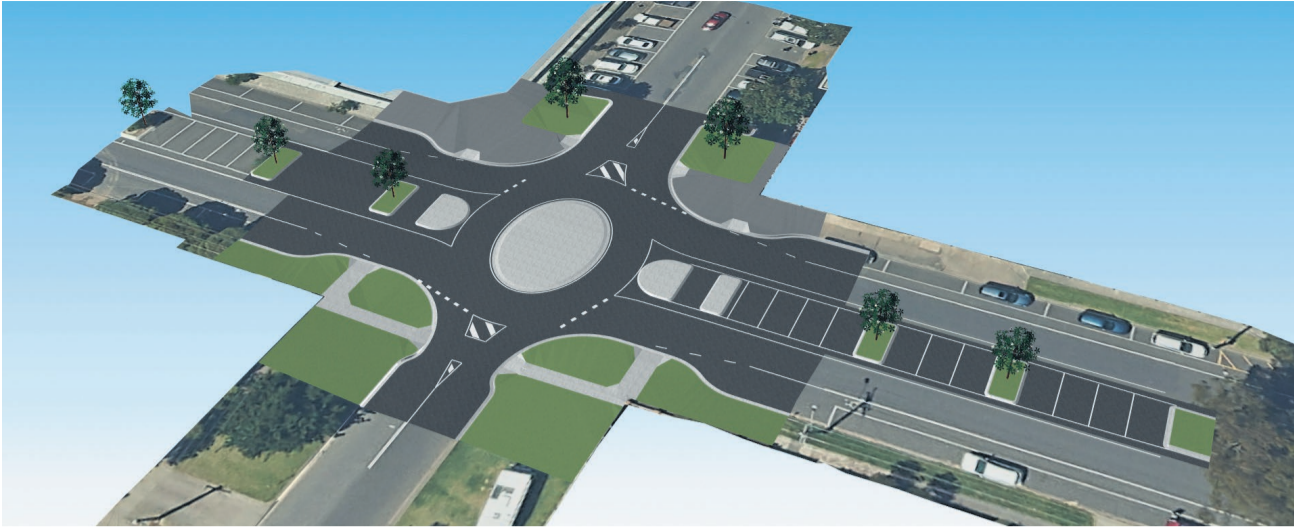
The new roundabout at the Desailly St and Macarthur St intersection roundabout will result in 10 additional carparks.
